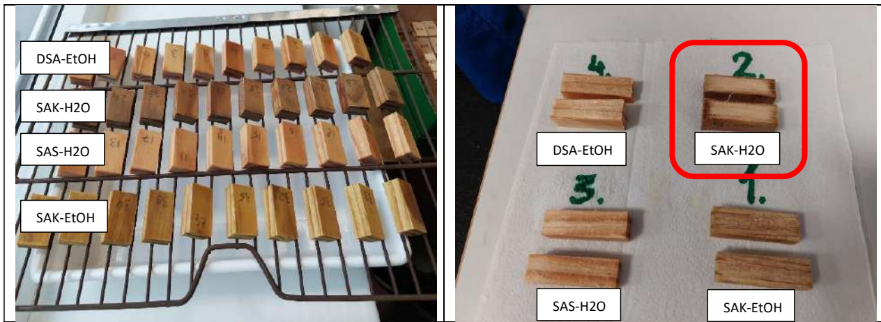
Fig.4. Wood blocks after impregnation prepared for drying (left) and cut samples (right)
